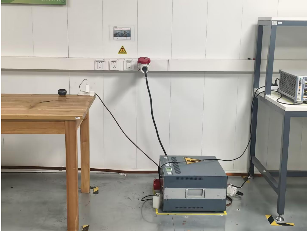
Photo of Power Line Conducted Measurement
