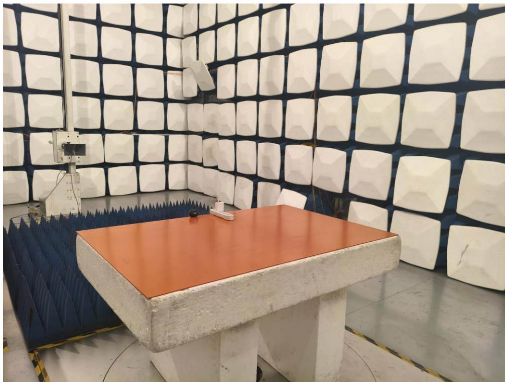
Photo of Radiated Measurement (Above 1GHz)
