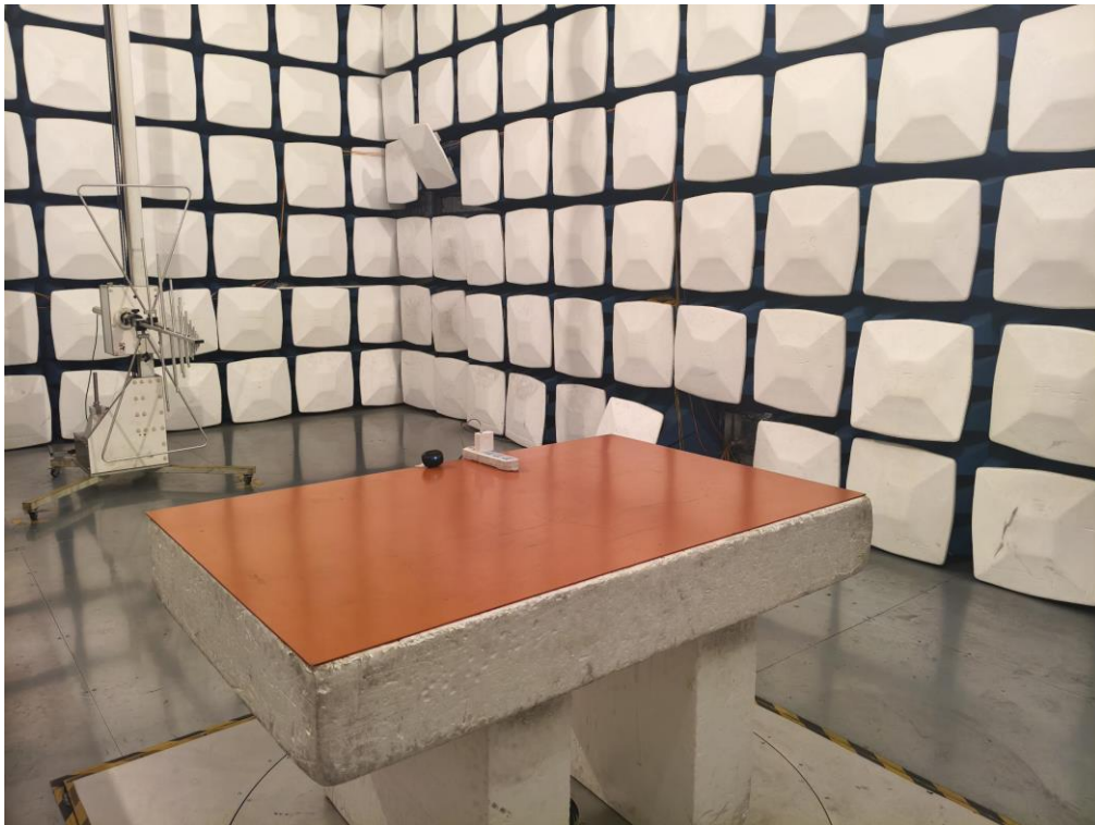
Photo of Radiated Measurement(Below 1GHz)
